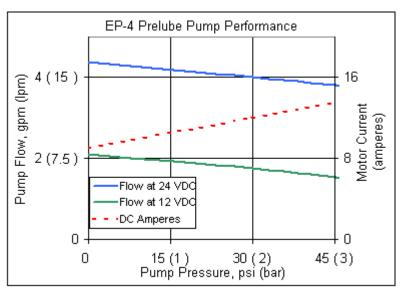
**Chart 1**- Pump Performance, Pump Flow as a function of Pressure.
