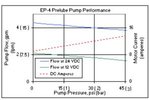
Nominal current draw for the EP-4 pump motor is 15 amps. Motor current varies with pressure. The motor should be fused. See wiring considerations.
