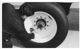
Figure 2. Check air pressure in tires
