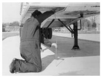
Figure 5. Measure from ground to kingpin
