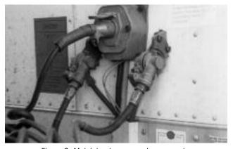
Figure 3. Maintain air pressure to suspension
