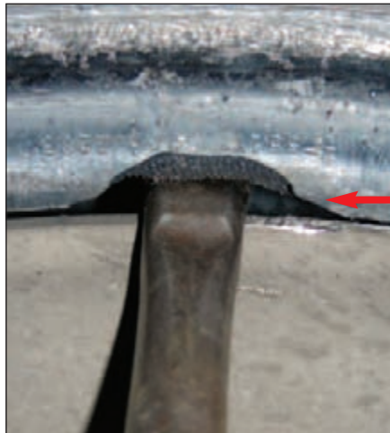
8 Failure to work with small sections on a non-lubricated bead will result in unnecessary damage to the bead.
