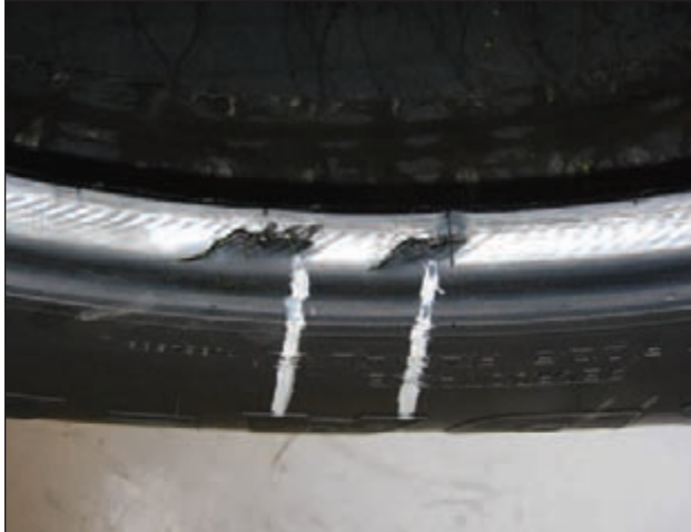
EFFECT: Heating and Deformation of the Bead Rubber CAUSE: Excessive Heat
