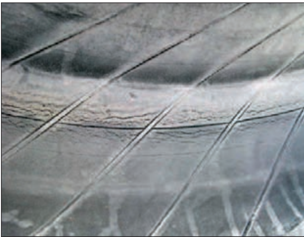
EFFECT: Inner Liner Cracking CAUSE: Underinflation
