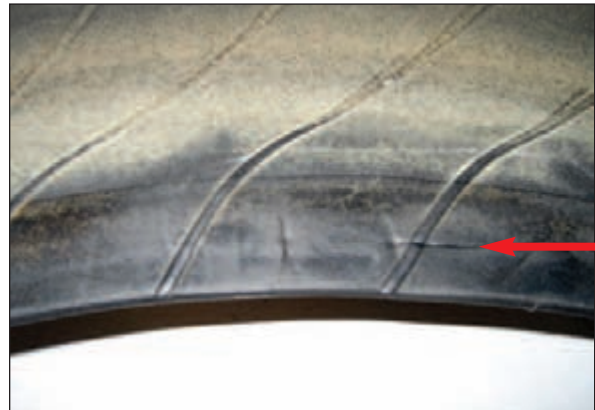
Severe inner liner damage from use of hammer.
