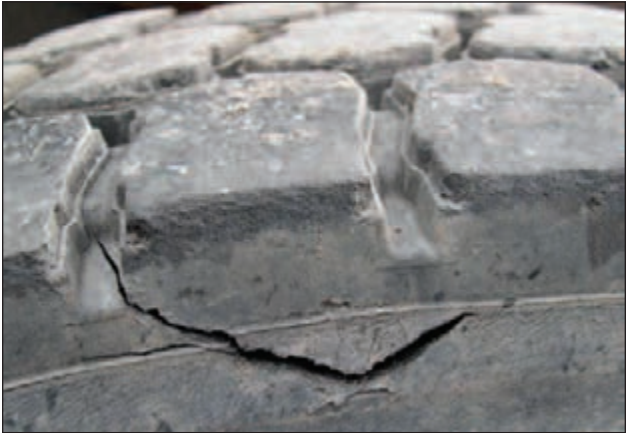
Sidewall Area Damage
