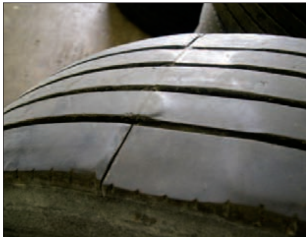
Open Splice Joint
