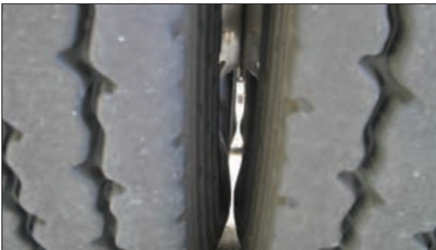
EFFECT: Friction Severely Weakens the Casing CAUSE: Improper Minimum Dual Spacing
