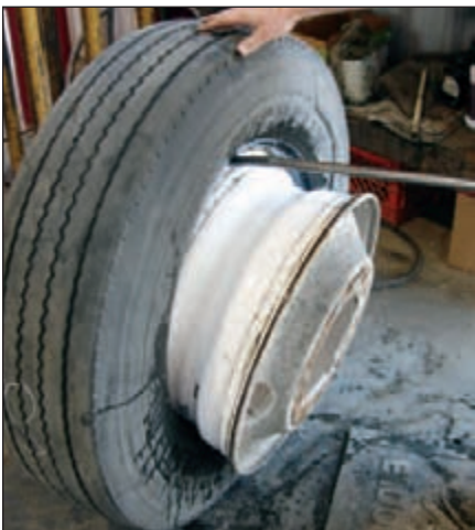
9 Lift the assembly, place the tire iron inside, rotate to lock the tab against the flange.
