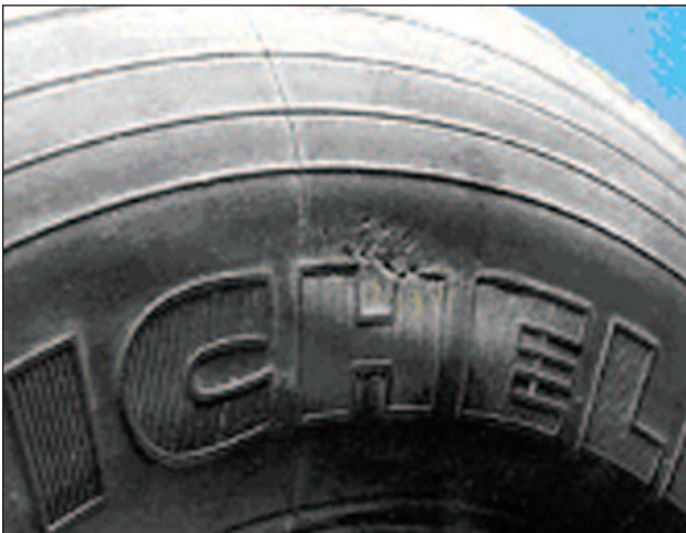
EFFECT: Small Bulge CAUSE: Impact With a Curb, Pothole, Road Debris, etc.
