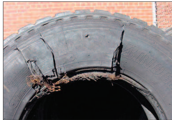
3rd Stage – Partial Unwrapping of the Casing Ply
