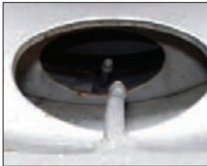
Incorrect Dual Wheel Placement
