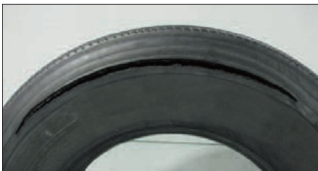
EFFECT: Zipper Rupture CAUSE: Damage/Weakening of Radial Steel Cables as a Result of Underinflation and Running the Tire Flat
