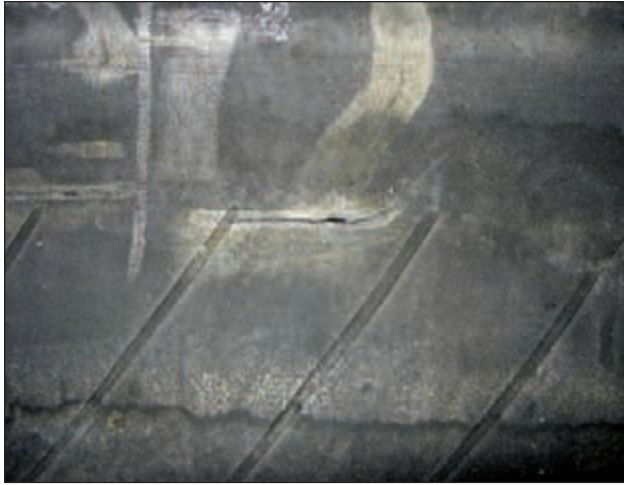
EFFECT: Inner Liner Cut CAUSE: Shipping or Mounting Damage
