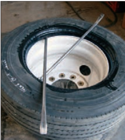
7 Completely unseat the first bead.
