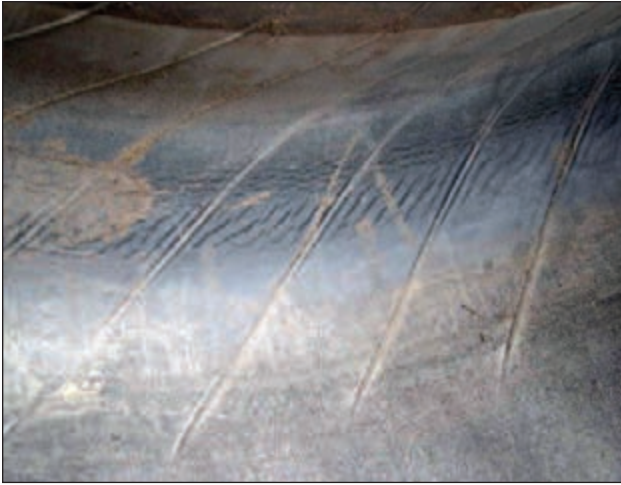
EFFECT: Inner Liner Marbling - Creasing CAUSE: Underinflation
