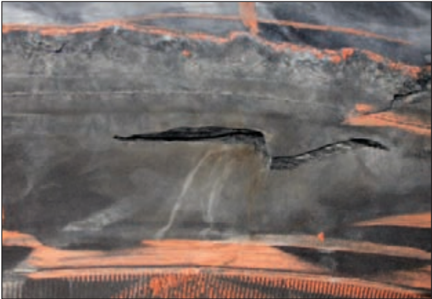
Sidewall Damage from Impact
