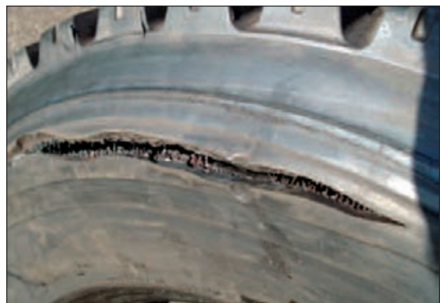
Zipper Resulting from Run-flat Condition
