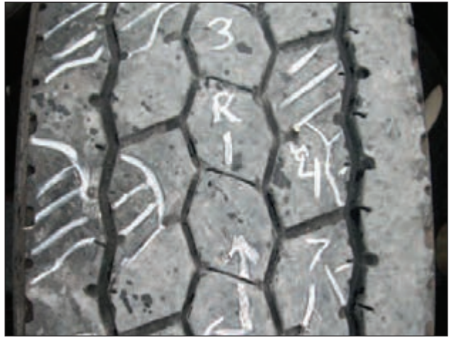
Cupping Wear – Drive
