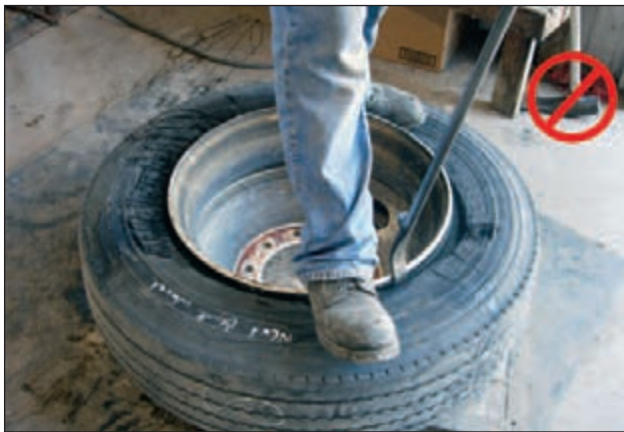
9 Use the proper tool, not the duck bill hammer .
