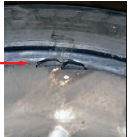
8 Failure to work with small sections on a non-lubricated bead will result in unnecessary damage to the bead.
