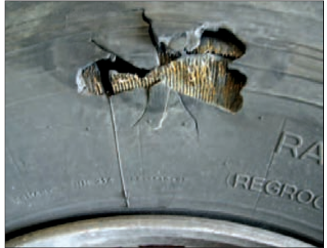
EFFECT: Impact Damage CAUSE: Severe Impact With Any Blunt Object
