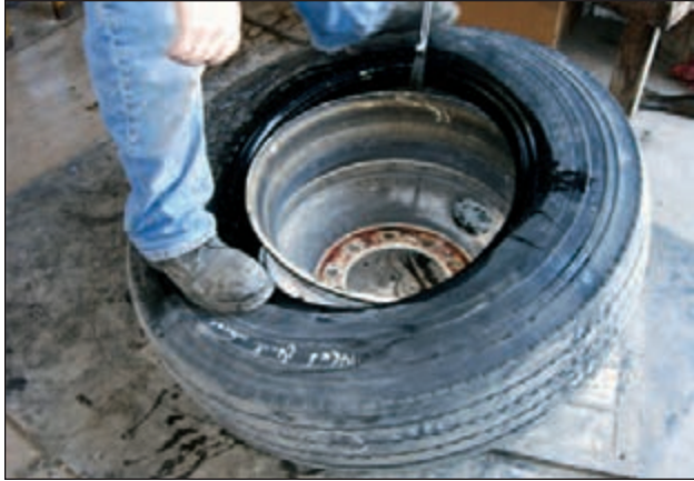
7 If necessary, continue to work the first bead on with proper tubeless tire tools.
