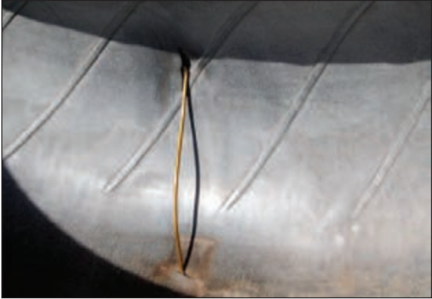
Example of sidewall penetration that damaged interior at crown. Road hazard damages should always be inspected on the inside and not repaired from the outside.
