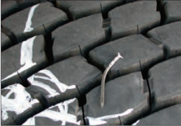
Inspect for Penetrating Objects
