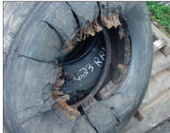
3rd Stage – Complete Unwrapping of the Casing Ply
