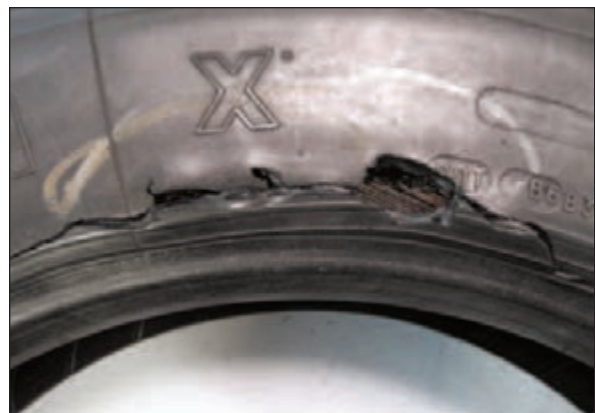
Resulting in sidewall separation and tire destruction from air infiltration.
