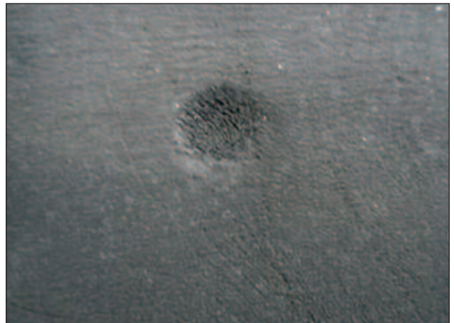
Worn Sidewall Depth Indicators
