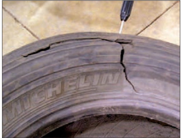
EFFECT: Crown/Sidewall Injury Resulting in Gas Loss CAUSE: Nail Hole Bolt/Debris Penetrating the Liner
