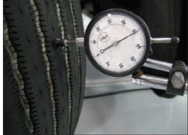
Measuring Radial Runout on Center Rib
