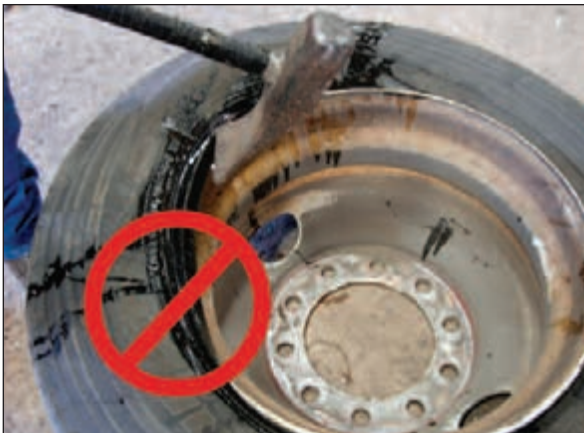
Do not use a duck bill hammer to seat either bead at mounting.
