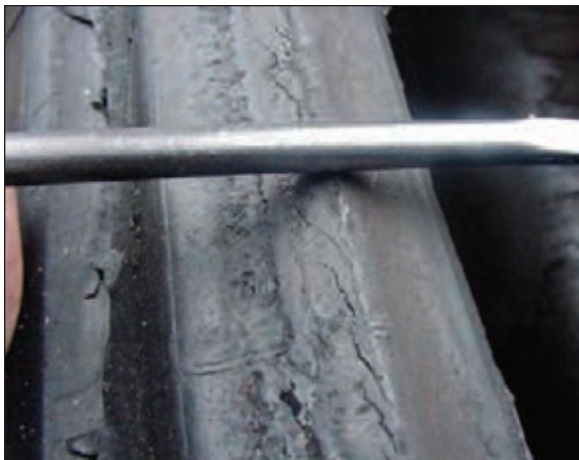
1st Stage – Turning of the Bead
