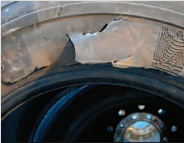
EFFECT: External Rubber Damage CAUSE: Severe Impact
