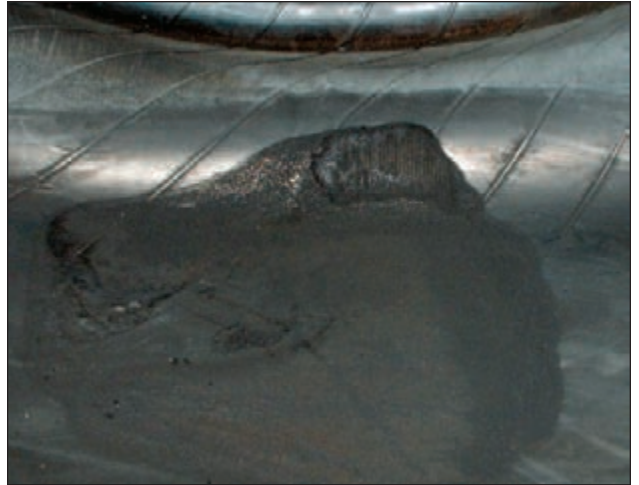
EFFECT: Inner Liner Burn CAUSE: Electrical Discharge Damage
