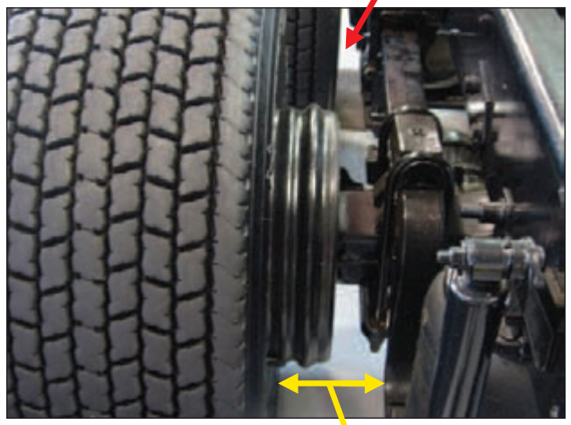
Correct Lateral Clearance
