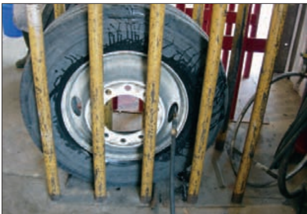
11 Place the assembly in the safety cage for safe inflation.
