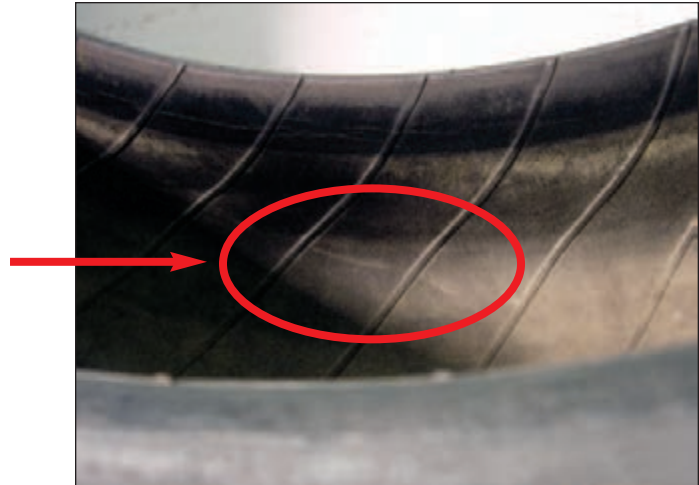
EFFECT: Internal Creasing CAUSE: Severe Impact
