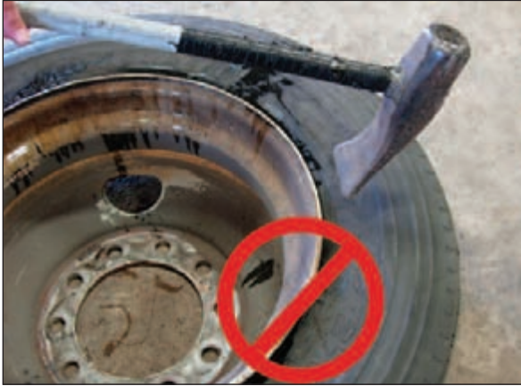
Do not use a duck bill hammer to break the bead at demount.
