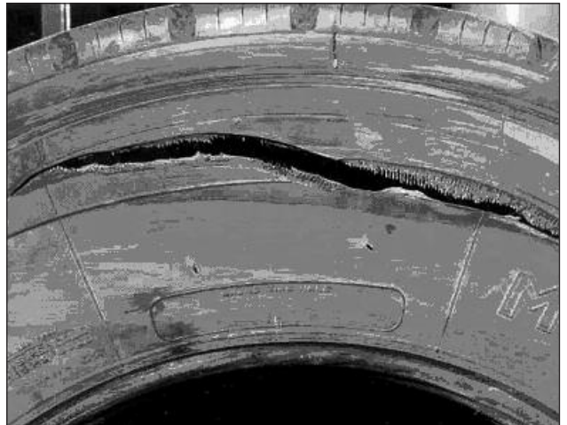
EFFECT: Impact Damage CAUSE: Sidewall Rupture from Shock
