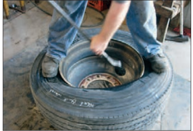
8 Mount second bead using same method.
