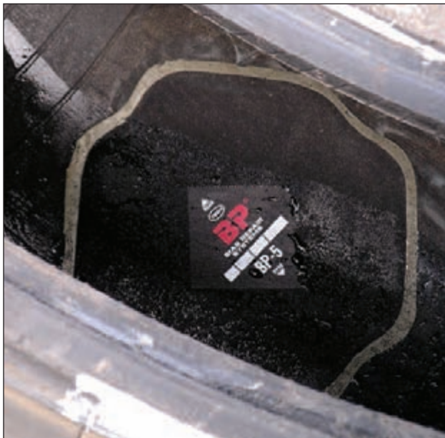
Improper Repair, Bias Ply Patch In a Radial Tire, Note Also the Misalignment
