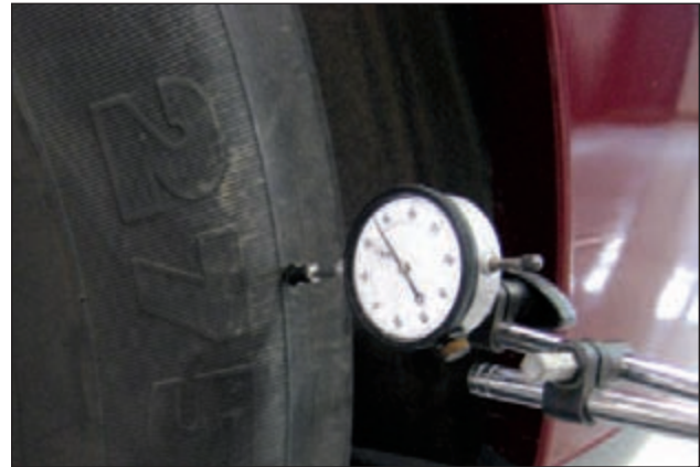
Measuring Lateral Runout on Outside Shoulder
