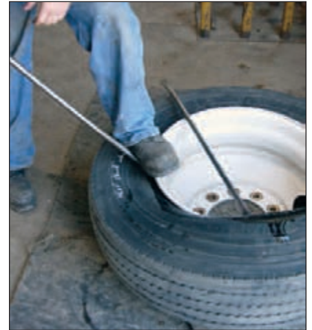
6 Progressively work tools around the wheel until the first bead is off the wheel.
