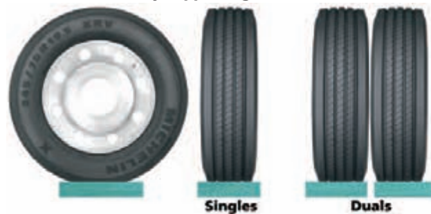
Correct Evenly supporting the full load.
