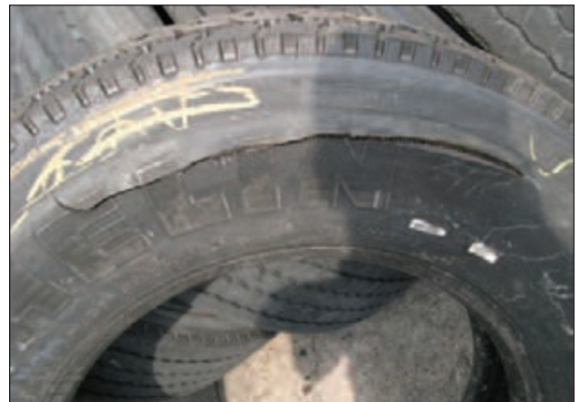
Fatigue Rupture or “Zipper”
