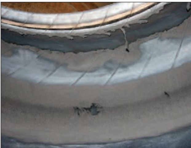
EFFECT: Discoloration, Blistering, and/or Separations of the Inner Liner CAUSE: Continued Operation After Loss of Inflation Pressure
