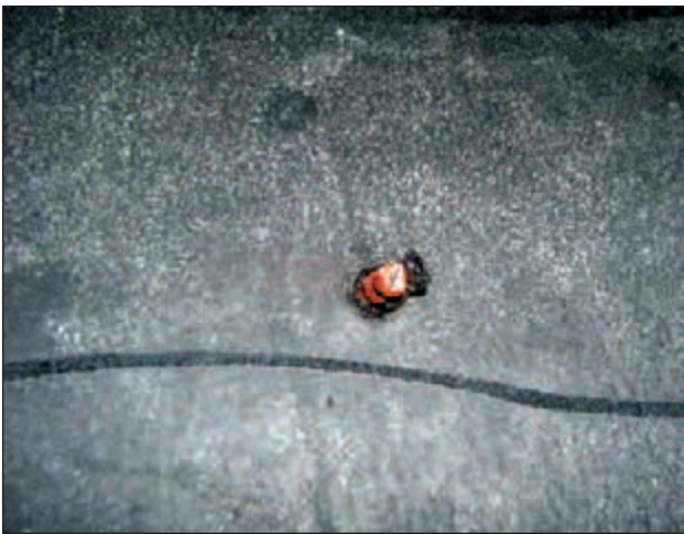
EFFECT: Premature Failure of Repair CAUSE: Object that Penetrates Into the Tire and Through the Inner Liner
