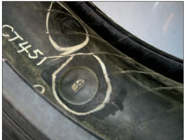
EFFECT: Improper/Incomplete Repair CAUSE: Internal Sidewall Damage from Penetrating Object Not Repaired
