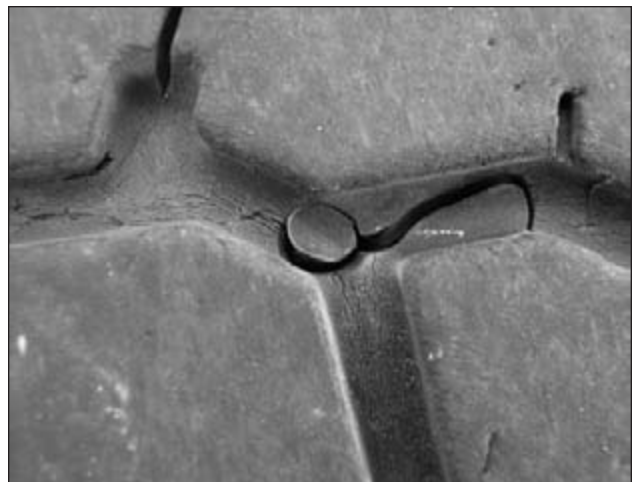
EFFECT: Crack Around Nail Hole Plug CAUSE: Improper Repair or Improper Repair Procedures
