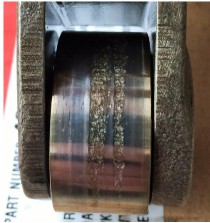
Galling and spalling on the exhaust roller and camshaft lobe
