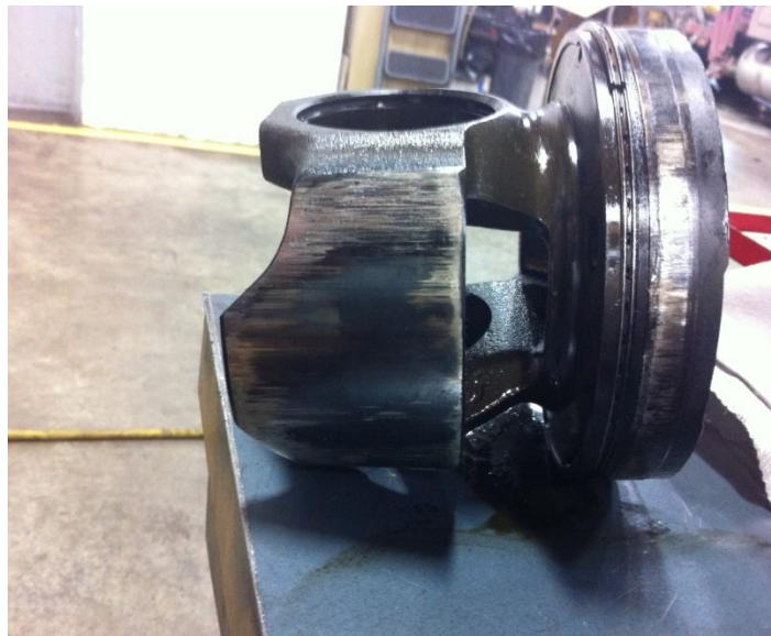
Cummins ISX piston with EGR at Pittsburgh Power The rings are stuck from soot and carbon causing it to destroy itself
