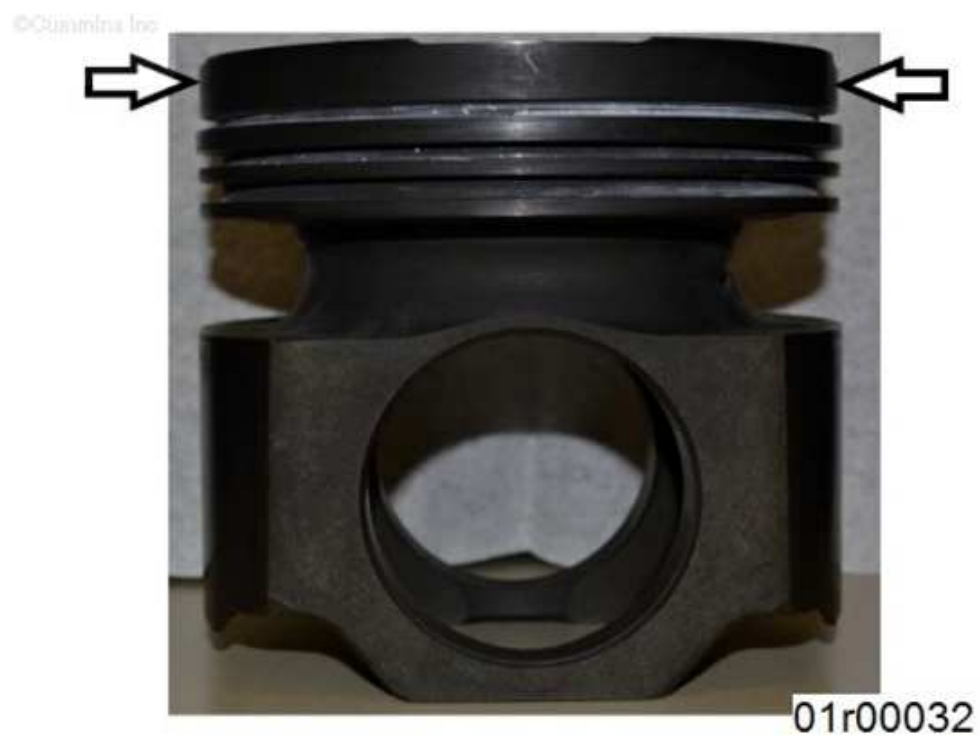
Figure 5, Measurement location to identify piston top land diameter
