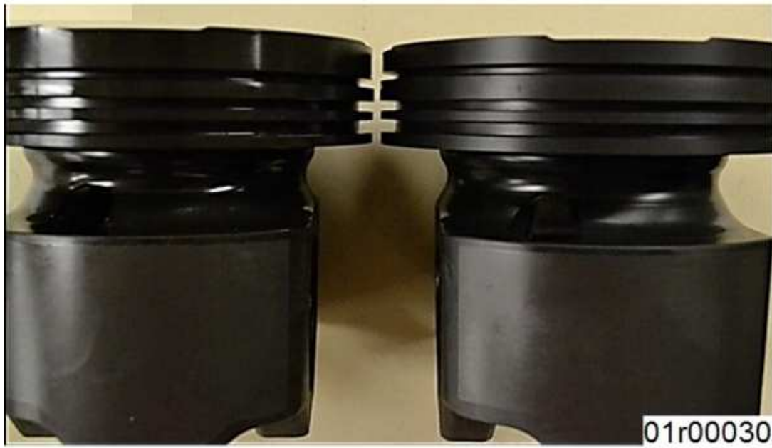
Figure 3, Low top ring piston on the left and a high top ring piston on the right
